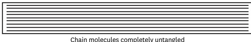
When fully stretched, they are all lined up (Figure 1(c)). At this point the rubber changes its appearance – the surface looks rougher and whiter.
