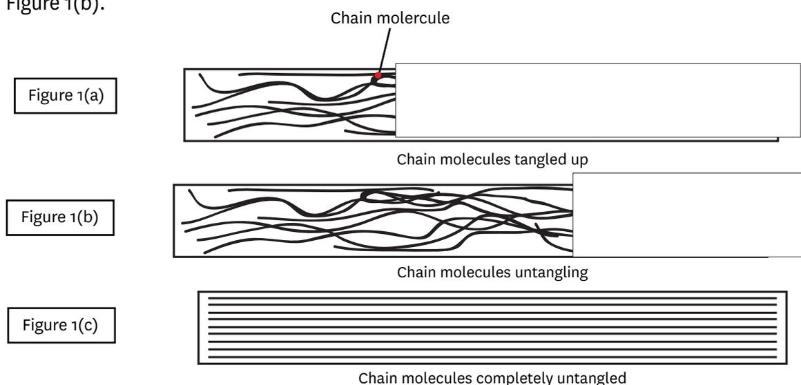
When fully stretched, they are all lined up (Figure 1(c)). At this point the rubber changes its appearance – the surface looks rougher and whiter.
